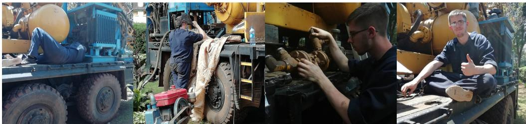
The support truck had failed to start, requiring a replacement starter relay / solenoid. In addition, the 25hp diesel motor for the welder was found to be running at about 50% required power which also explained the struggles for the crane and mini compressor to function efficiently. After servicing the injectors and replacing the leaking primer pump, it was still smoking badly and requires new piston rings from the UK.
